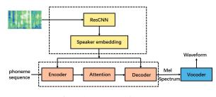
Figure 1: System architecture.
